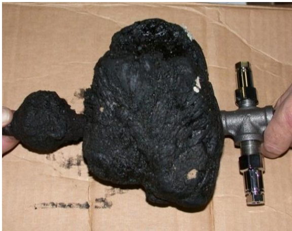
A comparison of block of grease on left to what is under the grease on right. This was the duct protection above a charbroiler. This picture was taken just after the fire-extinguishing system was allegedly serviced.
