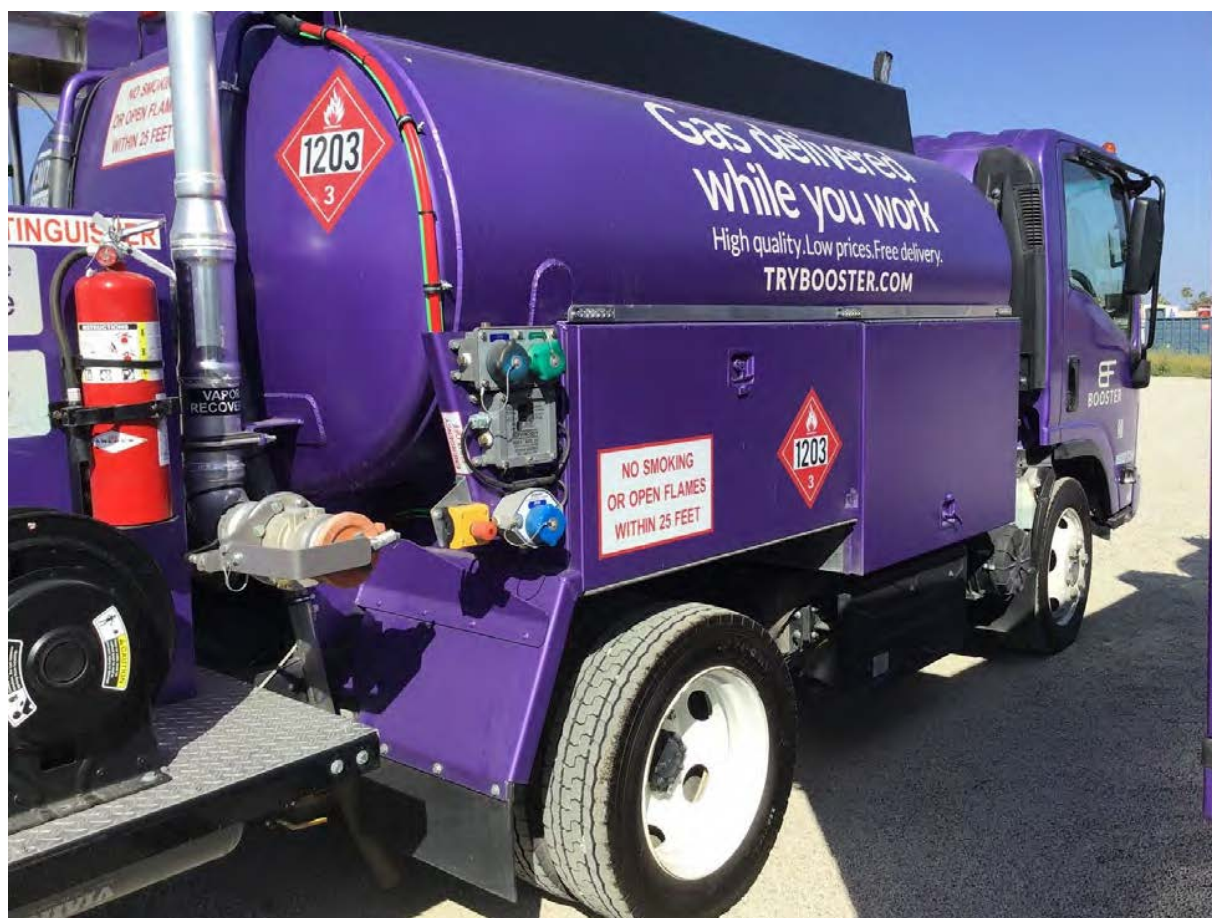
EXHIBIT J-Photo Of Approved Fire Extinguisher on a Booster Truck
